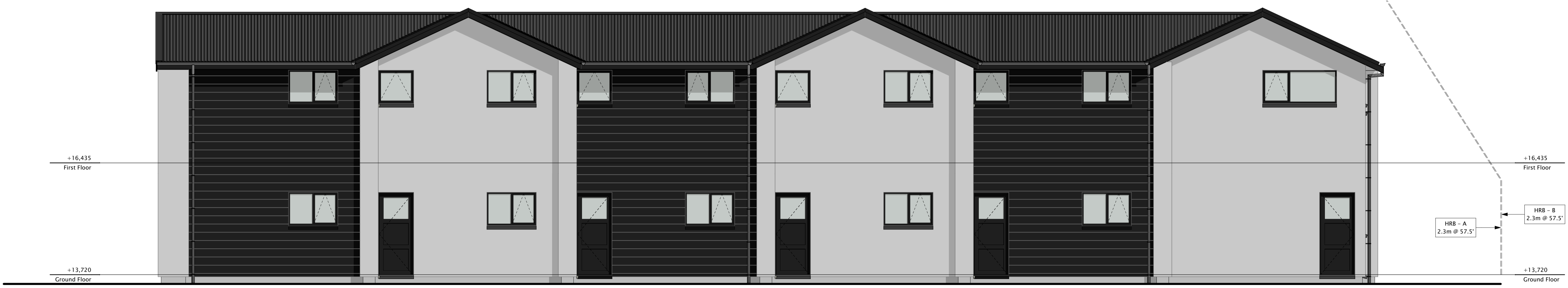
Units 1-6 South Elevation 1:50
