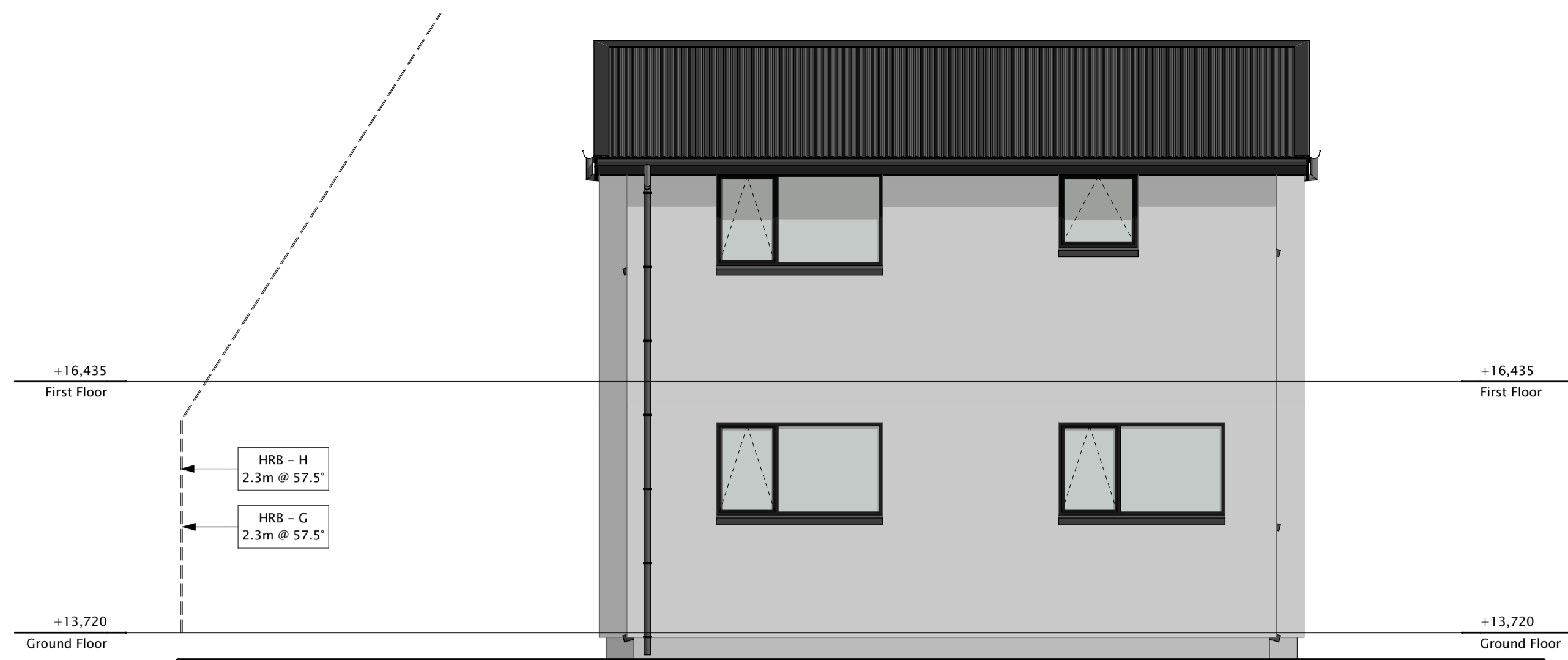
Units 19-21 North Elevation 1:50
