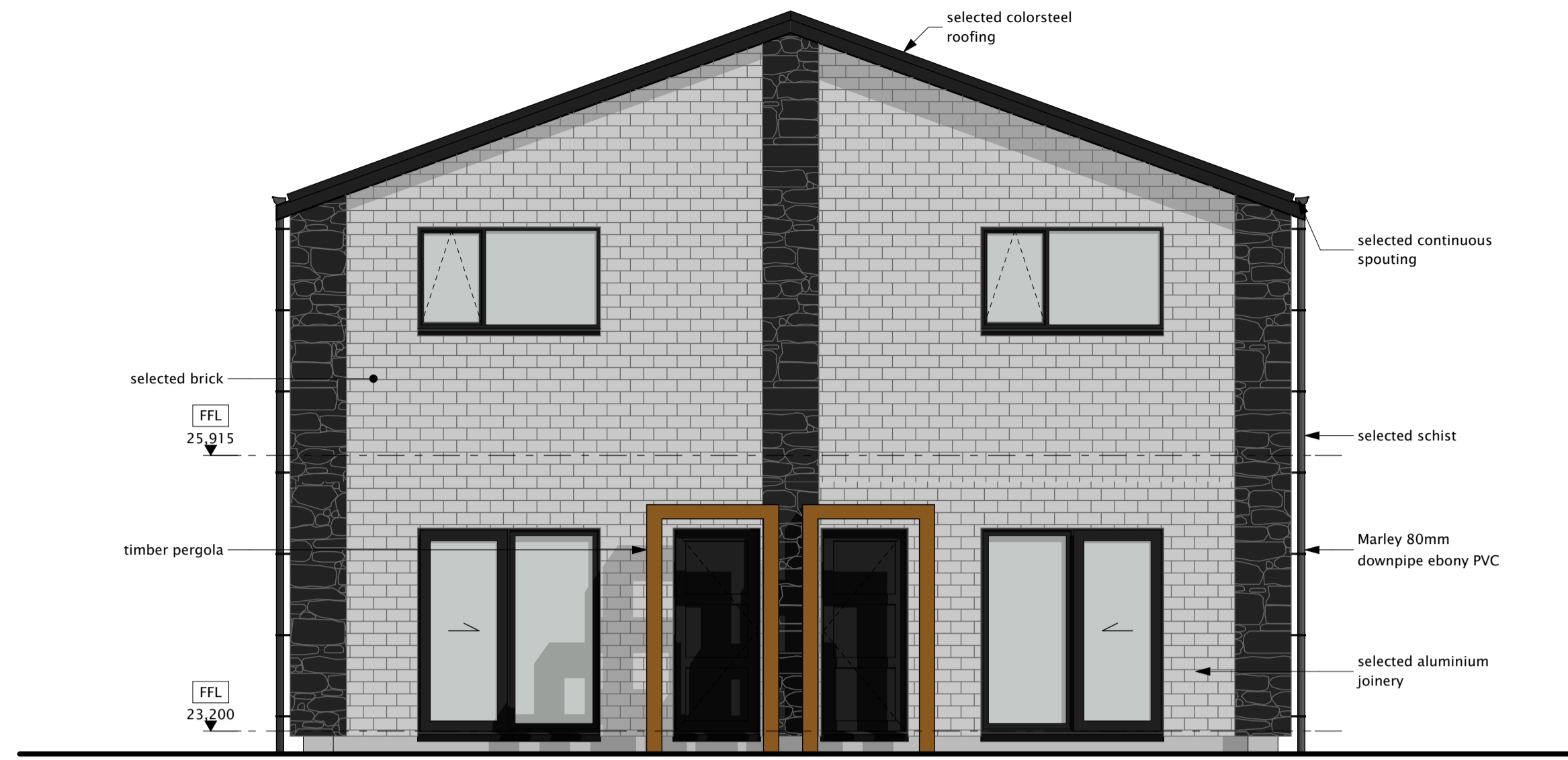
Units 1-2 North Elevation 1:50
