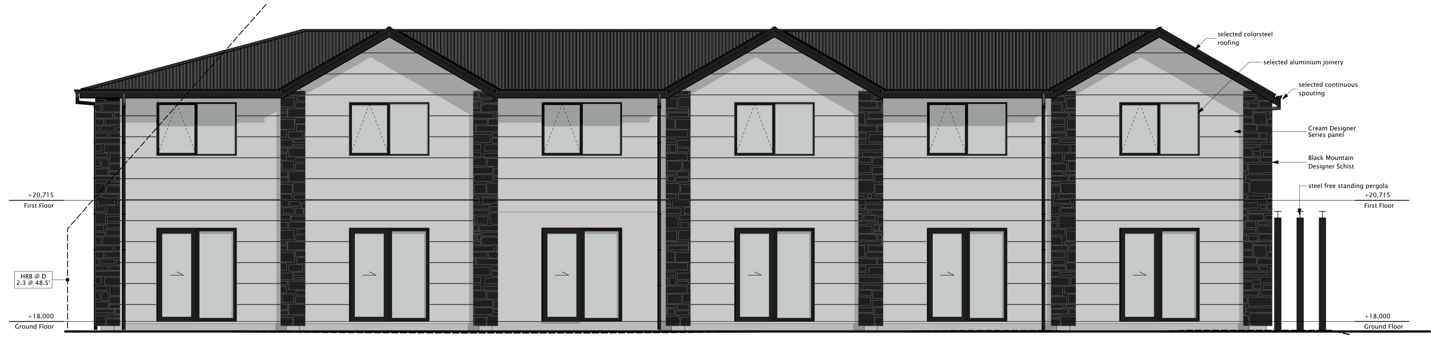
Brockworth Units 5-10 North Elevation 1:50
