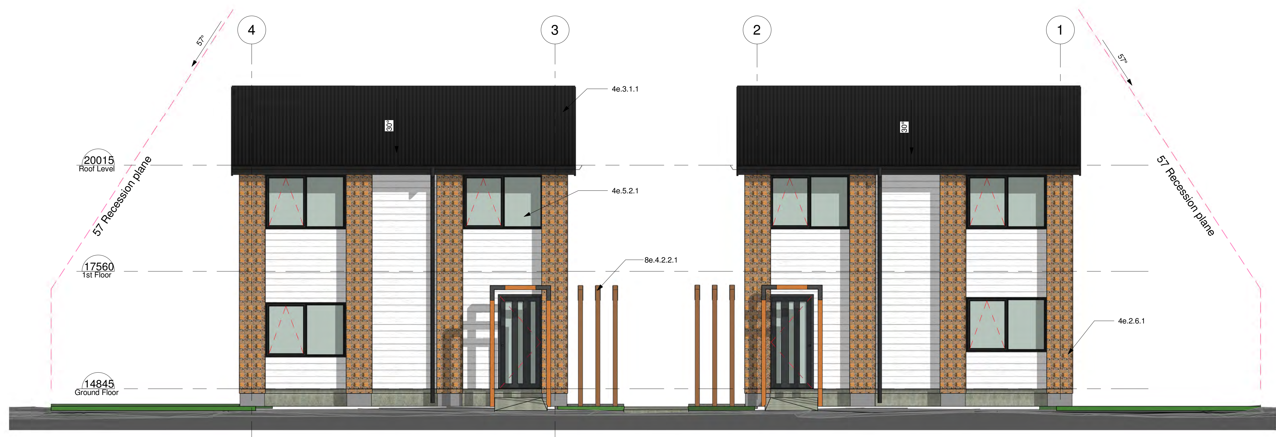
1 North Elevations Units 1 & 8 1 : 50
